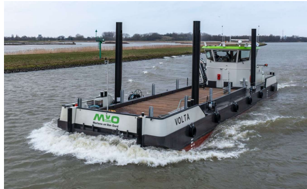
Werkship Volta (33,60 x 7,84 m, 2.200 kWh)
